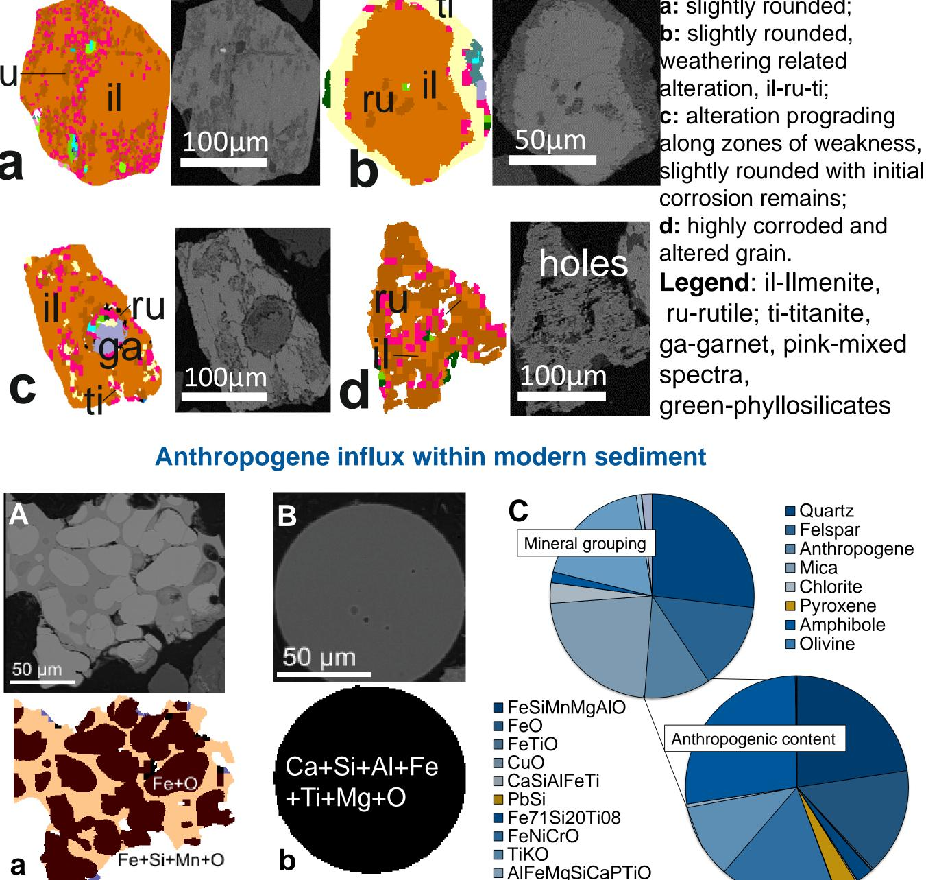
Figure description: Identification anthropogenic phases, to approximate and deduct the anthropogenic contamination. BSE (A,B) and false color (a,b) pictures of the anthropogenic contamination; chemical composition (provided by EDS). Based on these measurements the composition and amount of the contamination within one Sample can be calculated (**C**).
